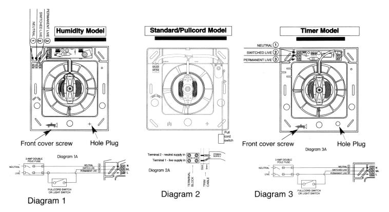
Important: Switch off mains supply before making any electrical connections. NB: Fan should be mounted at a minimum height of 2.2m. Fans should be installed by fixed wiring only. A flexible cord should not be used. Precautions must be taken to avoid the back-flow of gases into the room from the open flue of gas or other open-fire appliances when mounted in outside windows or walls.
