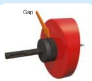
Screw the knurled ring clockwise to locate adaptor drive pins into the holes on the back of the holesaw. Notice the gap between the holesaw and the adaptor. This is necessary to prevent the holesaw locking onto the adaptor during the drilling process.
