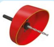
On the back plate of the holesaw are 4 drive pin location holes situated around the adaptor screw thread hole. The hole saw should be 'backed off' until the first pair of drive pin location holes line up with the adaptor drive pins.
