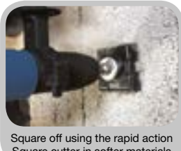
Square off using the rapid action Square cutter in softer materials
