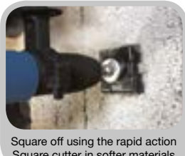
Square off using the rapid action Square cutter in softer materials
