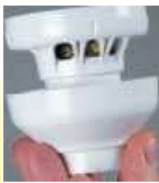
Cover Removal Cover can be completely removed after alignment.
