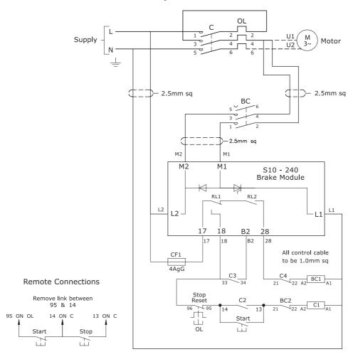
**NOTE:** On braking there is a diode in the brake circuit connected directly across the motor. Single phase induction motors have capacitors, permanent capacitors can be dc injected and the diode needs to be rated for the discharge currents of the motor capacitors this current can also produce a torque pulse on the shaft.
