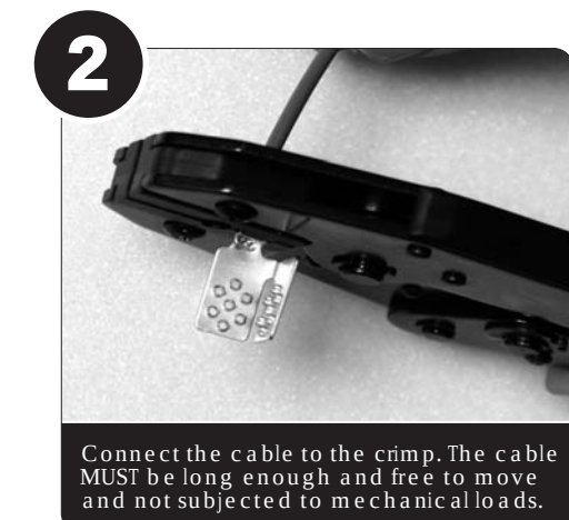
Bare the supply cable 6mm, and insert singly or in pairs into the cylindrical ferrule of the crimp connector
