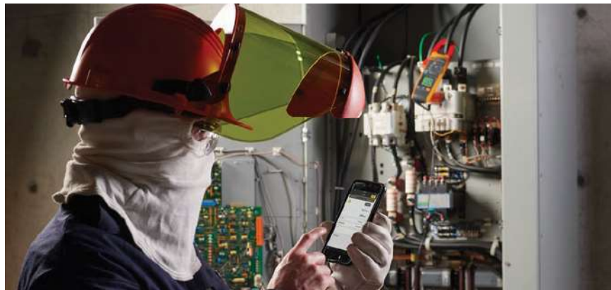
Fluke Connect allows measurements to be sent to a smartphone for logging, collaboration and analysis.
