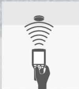
Upload settings to sensor – the luminaire blinks to confirm
