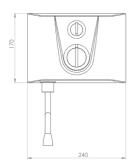
Outer Casing Easy clean, high impact polycarbonate/ ABS
