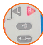
Rotary Field Indication, Continuity & Low Impedance
