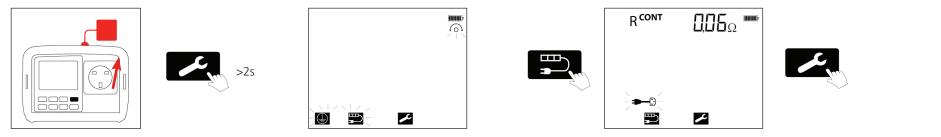
To NULL the resistance of the P1 continuity test lead
