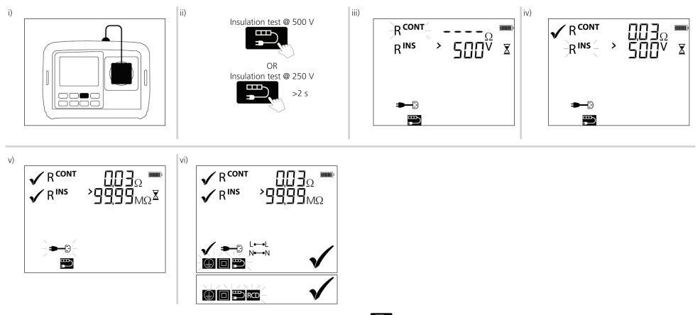
NOTE : For power cords longer than 5m the test can be re-run with a 1.0Ω pass limit by pressing the 😰 test button with 5 seconds of the continuity test failing – refer to page 13
