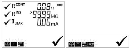
**NOTE 1**: If the contact symbol appears, the appliance needs to be switched ON. **NOTE**: The PAT100 instruments perform various pre-checks prior to testing to ensure the asset is not short-circuit and is switched on
