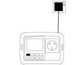
Connect the Instrument to the mains supply using the mains plug test lead (for mains powered leakage and RCD testing)
