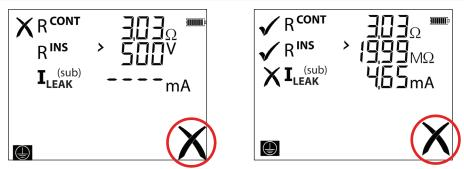
NOTE : Once an appliance has failed a test, further testing of the test group sequence is prevented for safety reasons, except for the extension lead testing
