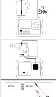
Connect the P1 test lead to socket P1 on the Pat100 and the probe to exposed metalwork Ensure the probe is NOT connected to a 230V source.
