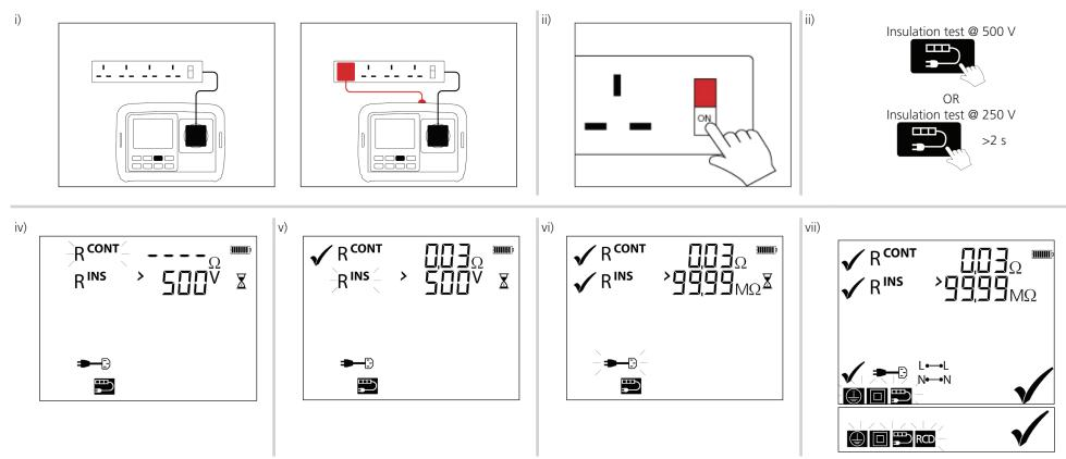
NOTE: Multiple earth continuity tests can be carried out by pressing the QT button during the continuity test, and pressing it again for each new continuity test. See Page 13
