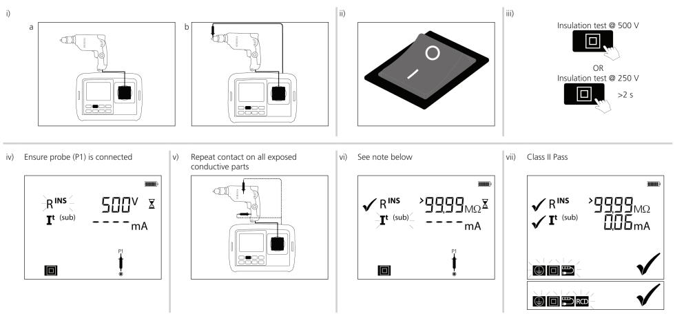
**NOTE:** If the contact symbol  $\stackrel{\checkmark}{\longrightarrow}$  appears, the appliance needs to be switched ON **NOTE**: The PAT100 instruments perform various pre-checks prior to testing to ensure the asset is not short-circuit and is switched on
