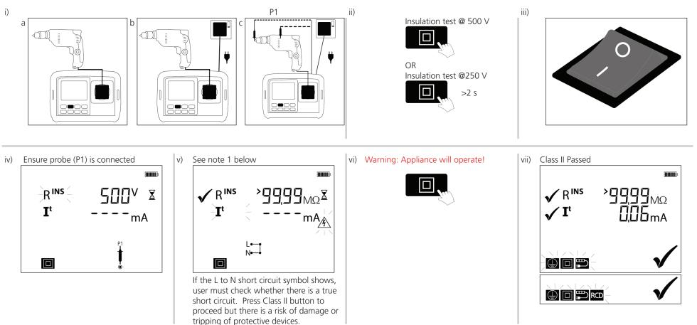
NOTE : High touch leakage measurement on faulty equipment can trip the supply RCD
