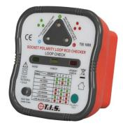
The TIS 1005 is a pocket sized checker for indicating loop impedance, socket polarity and RCD 30mA are all ok. Indication is by LED's and buzzer. It is an ideal unit for initial "checking out" of a 13A socket and will advise if the circuit is ok, needs attention, or needs urgent attention. An ideal product for housing associations, landlords, council property departments, shopping centres, electricians etc.
