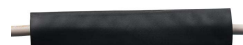
The shrink tube must have an overlap length of at least 30 mm on the cable sheath.
