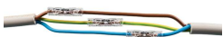
Strip 10 mm conductor per specification and insert connector (example shows staggered connectors).
